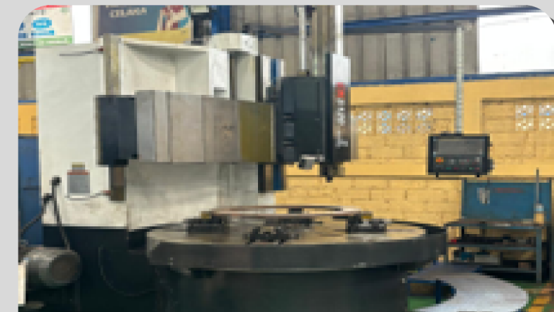
CNC Vertical Lathe Max Ø2000mm
